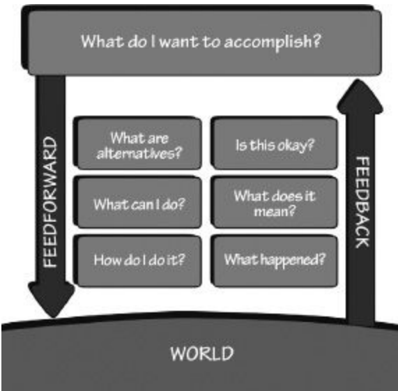
FIGURE 2.7. The Seven Stages of Action as Design Aids. Each of the seven stages indicates a place where the person using the system has a question. The seven questions pose seven design themes. How should the design convey the information required to answer the user's question? Through appropriate constraint and mappings, signifiers and conceptual models, feedback and visibility. The information that helps answer questions of execution (doing) is feedforward . The information that aids in understanding what has happened is feedback .
