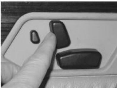
FIGURE 1.7. Good Mapping: Automobile Seat Adjustment Control. This is an excellent example of natural mapping. The control is in the shape of the seat itself: the mapping is straightforward. To move the front edge of the seat higher, lift up on the front part of the button. To make the seat back recline, move the button back. The
