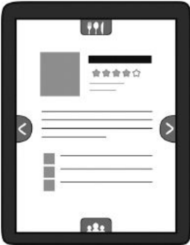
FIGURE 1.6. Signifiers on a Touch Screen. The arrows and icons are signifiers: they provide signals about the permissible operations for this restaurant guide. Swiping left or right brings up new restaurant recommendations. Swiping up reveals the menu for the restaurant being displayed; swiping down, friends who recommend the restaurant.
